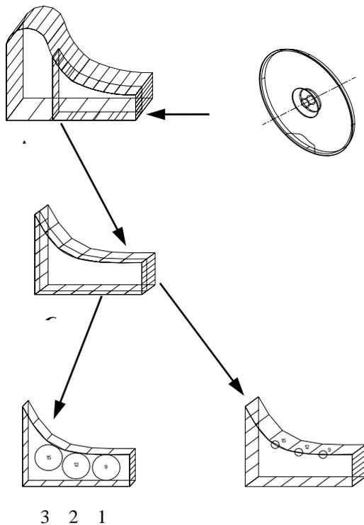
Fig. 8. Schematic of cutting of specimens
