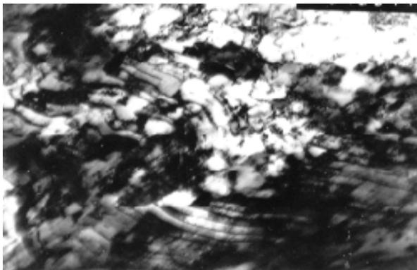
Fig. 9. Fragmentation of structure in the dominant work hardening zone
