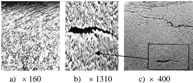
Fig. 5. Ferrite-carbide mixture with a deformation texture (a), expanded non-metallic inclusion (b) and surface microcrack (c)
